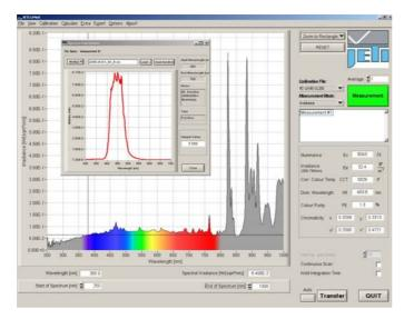
Screenshot of a Xe lamp spectrum, inserted is a spectrum weighted with the function of the photochemical injury caused to the eye by blue light radiation ( $B(\lambda)$ )
