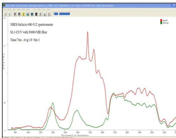
**RED-Wave-NIRx-SR-InGaAs-512 spectrum showing % Transmission data of alcohol and oil samples for 900-2200nm range. Data obtained with SL1-CUV which is an integrated halogen light source + cuvette holder.**
