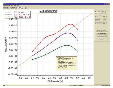
Single-Sine experiments acquire an impedance spectrum over a range of frequencies (range is instrument-dependent) with the cell under potentiostatic control in two, three, or four electrode configurations. The user can control the AC voltage amplitude, DC bias voltage, starting and ending frequencies, number of data points sampled (linear or logarithmic), and measurement delays.
